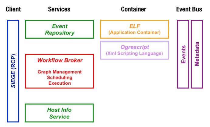
The principal mode of access is through our Eclipse-based RCP client, Siege. The service layer currently consists of the main service, the Workflow Broker, plus the Host Information Service and Event Repository. The container used for managing jobs on hosts is Elf, with its native scripting language, Ogrescript.
